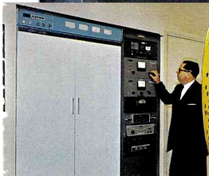
The new 10KW Gates FM 10-G transmitter brings listeners true "color" fidelity — rich sound with delicate gradations of tone. This transmitter is "on the air" at KTRH, Houston, Texas.
